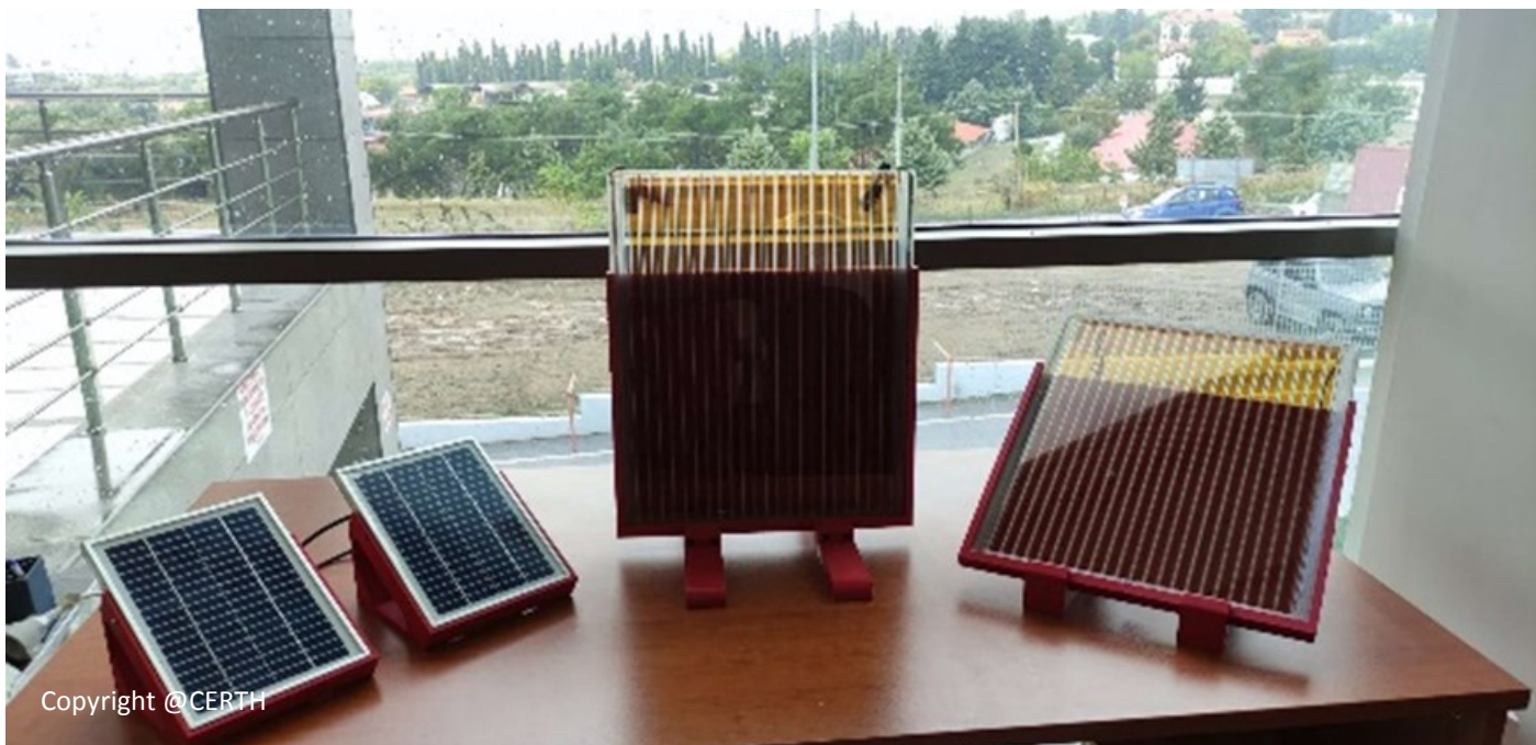
3D printed cases for the pVs
